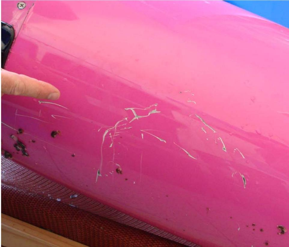
Fig. 3. A likely shark bite (~15 cm diameter) on the ocean-scarred glider.
